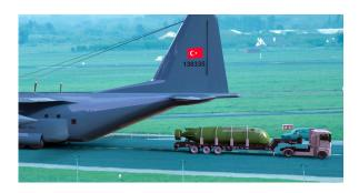
**DATUM DRY COMBAT SUBMERSIBLE** is a dry swimmer delivery vehicle, which can be transported inside a standard 40 foot container. This allows a transport inside a ship container via sea, air or land transportation covertly. Vehicle can carry up to 8 combat swimmers while two of them are enough for the operation of the craft. Thanks to the diver lockout chamber inside, it can dry transport combat swimmers and carry up to two wet type swimmer delivery vehicles.
